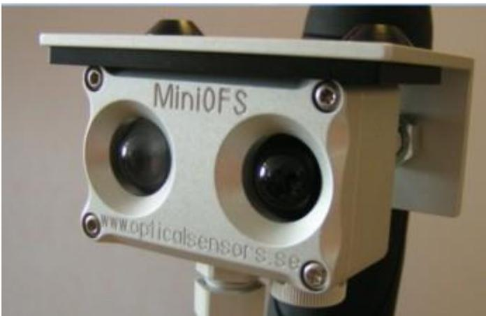
The sensor is sensitive for particles in a zone about 25 cm ahead of the location of the sensor that limit the visibility in the air. These particles are normally the microscopic water particles constituting fog, but they may also be snowflakes, raindrops or air pollutants. But the particle density must be high enough to limit the visibility to lower than about 2000 meters. The sensor is heated to a few degrees above ambient temperature in order to keep moisture away
